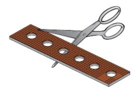
**Step 1**: Cut the strip into pieces of desired length (Only required when the product is delivered as strip)
