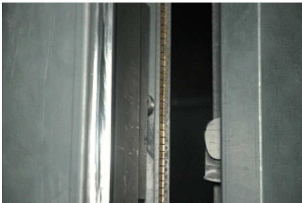
Heavy-duty fingerstrip sliding door locking mechanism
