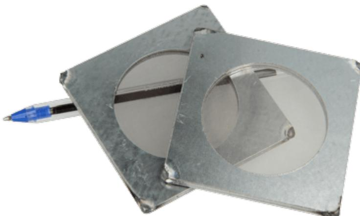
Mesh clamped between 2 plates, welded on corners
