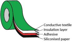
Our conductive textile tape with adhesive on the back can be supplied with a 0.15 mm thick white insulation layer or with a 0.22 mm thick black one, and can be delivered on rolls.
