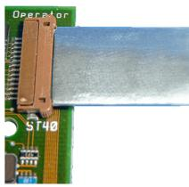
Ready-made sleeve for flat cable. The sleeve is made from Amucor foil
