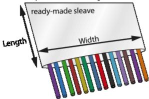
Technical drawing: How to specify the length andwidth of the ready-made cable shield
