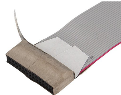
Step 1. Flat cable connector shield stuck on the connector
