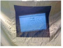
Conductive mesh can be used to create windows in for example a Faraday tent
