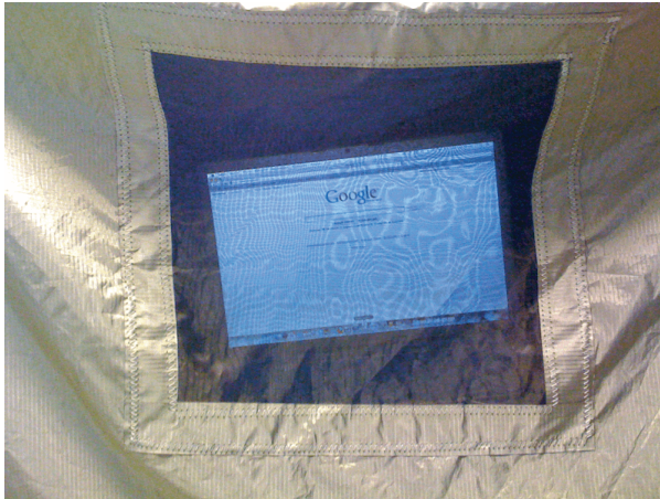
Shielded ventilation mesh
