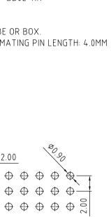
(Tolerance: ±0.05) RECOMMENDED PC BOARD HOLE LAYOUT
