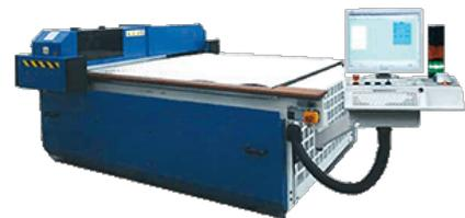
*With our automated CNC cutting system, we can cut Amucor foil in large quantities and according to your CAD drawing*
